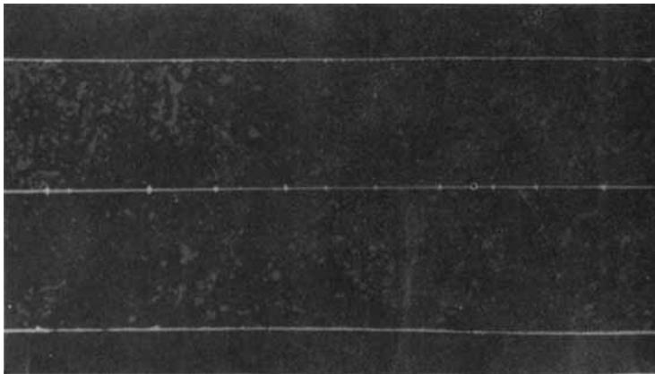
Fig. 3. Typical breaking pattern of a single fiber embedded in the epoxy resin. (Good bonding.)
